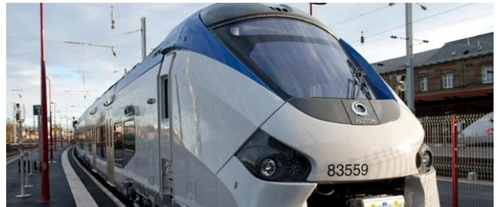
The reduced weight, traction system, associated with an original design of **Coradia Polyvalent** enable a reduction in energy consumption of around 15% compared to previous generations. The lifecycle of the trains, from their conception to their recycling, represents an investment for the future due to their very long lifespan. Coradia Polyvalent is over 98% recoverable.
