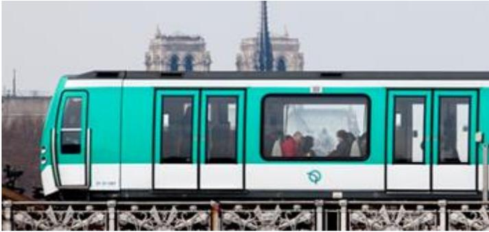
The braking system of the **new type of metro for the Paris network (MP14)** is 100% electric, recovers energy and injects it back into the network in the form of electricity, thus avoiding the emission of fine particles from brake pads. This system reduces air pollution as well as the metro's energy consumption by up to 20%.
