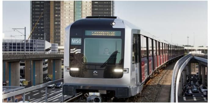
Despite its wide gauge, **the Metropolis train for Amsterdam** is low weight (12 tons per axle) thanks to its aluminium body and redesigned components. Its electric braking until the train comes to a complete stop enables full recovery of the braking energy and reduced dust and noise emissions. Its lighting is 100 percent LED. The Amsterdam metro is one of the quietest in the world (-8dB interior noise level).
