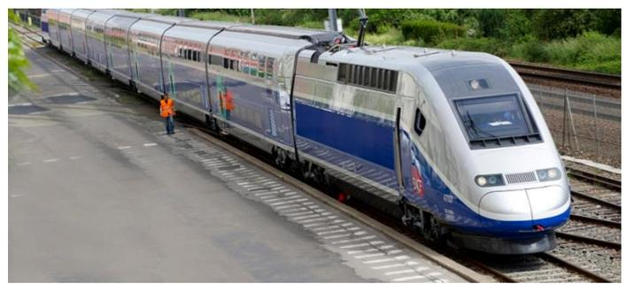
**The Euroduplex** is the only double-decker very high-speed train in the world. The consumption of energy per seat is 20% lower than in single-deckers and the trains can carry between 20% and 40% more passengers in high comfort.
