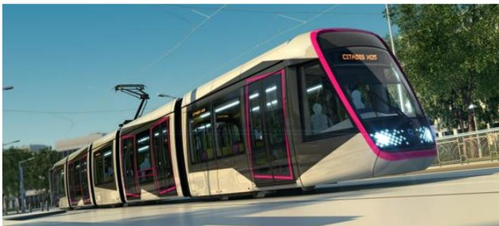
**Citadis trams** now include permanent magnet motors, an optimisation of the traction system to reduce energy consumption and making the trams highly recyclable by using materials designed to protect the environment. Since it first entered service, more than 5 million tonnes of CO<sub>2</sub> emissions have been avoided by Citadis operations.
