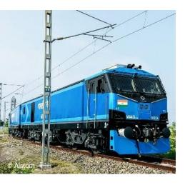
**19 May 2020** – The first of the 12000-horsepower, Prima T8 electric locomotives has been put into commercial service by Indian Railways. Built by Alstom and certified by the Ministry of Railways and Commissioner of Railway Safety/RDSO, the electric locomotives – known locally by the designation WAG-12 – are the most powerful locomotives to run on Indian rails. The 2015 contract will see a total of 800 locomotives built for Indian Railways.
