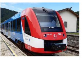
**11 September 2020** – In Vienna, a new era in passenger rail starts today. Until the end of November, a hydrogen train will run for the first time in regular passenger service for ÖBB, the Austrian Federal Railways. The Coradia iLint, built by Alstom in Salzgitter, Germany, uses on-board fuel cells to convert hydrogen and oxygen into electricity, thus reducing operating emissions to zero.
