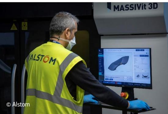
**May, 31, 2021** – The 3D Printing Hub at Alstom's Santa Perpètua Industrial Center, in Barcelona, opens new facilities in a space dedicated to the entire Alstom 3D printing team and equipment. The new facilities, located in the heart of the factory, has a component scanner, ten FDM<sup>1</sup> industrial wire machines, and three SLA-DLP<sup>2</sup> resin devices, which allow printing tools for industrial centers and prototypes to validate designs, moulds, and serial parts.
